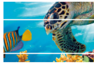
Gap/White streaks (Excessive feeding amount)
