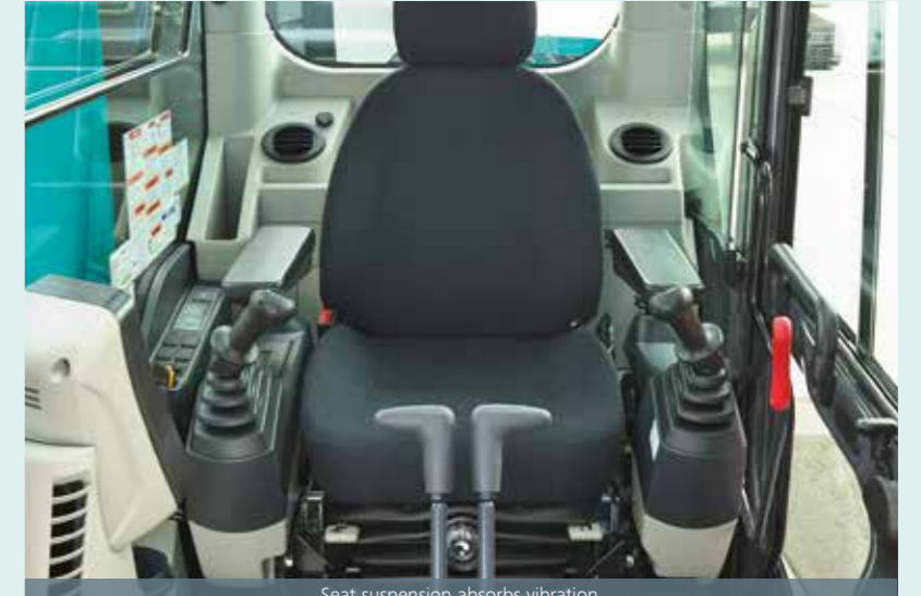
Seat suspension absorbs vibration
