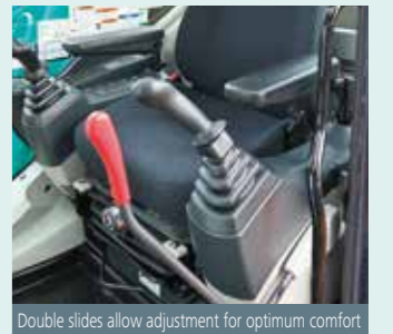
Double slides allow adjustment for optimum comfort
