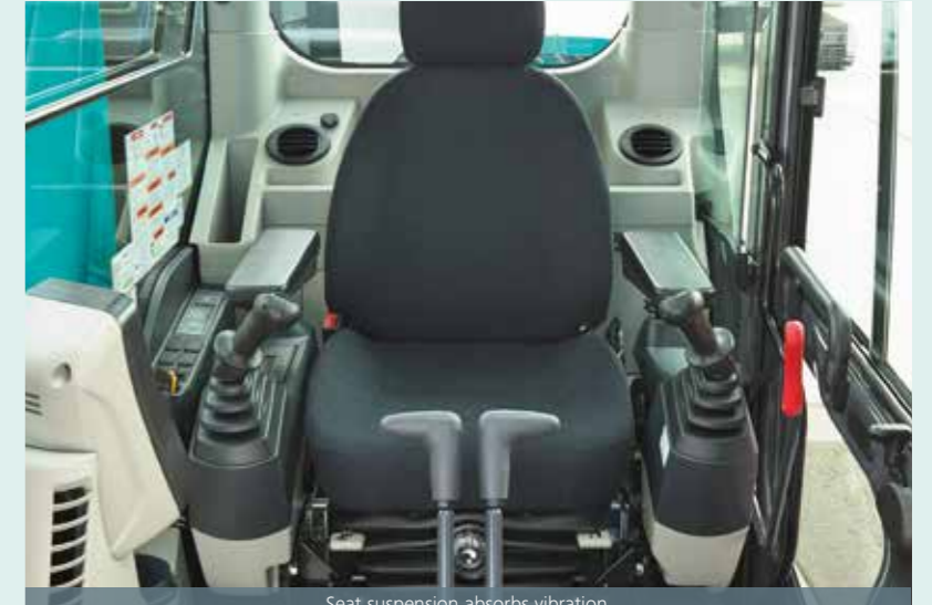
Seat suspension absorbs vibration
