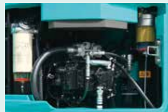
Fuel filter with built-in water-separator
