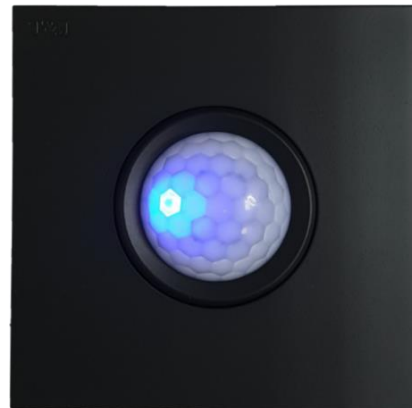
Motion sensor when triggered (blue LED lit up)
