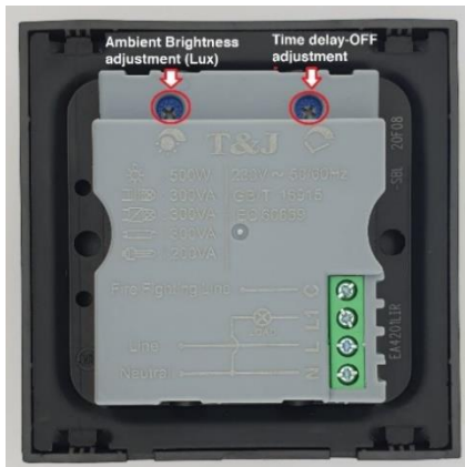
Motion sensor ambient brightness and time delay-off adjustments
