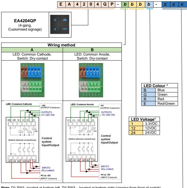
Note: D1,SW1- located at bottom-left, D3,SW3 - located at bottom-right (viewing from front of switch)
