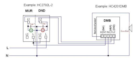
Cap.\* - Add 0.15uF/0.22uF,275VAC X2-Safety Capacitor across LED indicator if there is residue voltage issue
