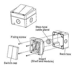
**Note:** When re-installing switch cap, observe orientation, left or right cap and in "up" position.
