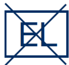
Lamp not suitable for emergency operation
