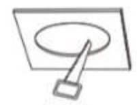
P-1 1. Open the hole as required size on the ceiling, as P-1.
