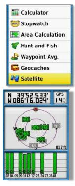
Access the *Satellite* page by going to the Main Menu (press Menu twice, or use Page and the ribbon menu to navigate to the Main Menu). When the Main Menu opens, it will default to the top of the list and the Setup menu will be highlighted. DO NOT enter the Setup Menu. Instead, press UP once on the Rocker button and the Main Menu will "wrap" to the end of the list and Satellite will be highlighted. Press Enter.
