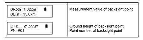
When the current measurement finishes, press  $[\blacktriangle]$  or  $[\blacktriangledown]$  to display the following screen.
