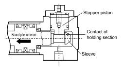
Inspect the piston once or twice a year to make sure there is no damage to the retainer caused by this phenomenon.
