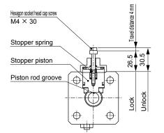
Manual override locking release method By rotating the round nut leftward (counterclockwise), the stopper piston moves and the lock is released. Rotating the round nut to the right (clockwise) to set it in the locked position causes the stopper piston to return. When it fits into the piston rod groove, the piston is locked.
