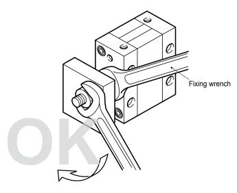
■ For female threads, fix the wrench hook at the end of the rod with a wrench using a standard tool (Allen wrench), and tighten.
