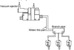
■ Perform piping with a sufficient effective crosssectional area. For the vacuum piping side, select a piping with sufficient effective cross-sectional area to allow the flow of the max. suction flow rate to the ejector. ■ When using MVC with reed switch, the cylinder cannot be mounted on a magnetic substance (iron plate, etc.). This could lead to switch detection malfunction.
