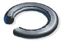
**Description:** The seal often exhibits discoloration, as well as powdered residue on the surface and possible erosion of elastomer in the exposed areas. **Contributing Factors:** Chemical reactivity of the plasma. Ion bombardment (sputtering). Electron bombardment (heating). Improper gland design. Incompatible seal material.
