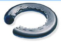
**Description:** The seal develops ragged edges (generally on the low-pressure side) which appear tattered. **Contributing Factors:** Excessive clearances. Excessive pressure. Low-
