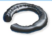
**Description:** The seal may exhibit many signs of degradation including blisters, cracks, voids or discoloration. In some cases, the degradation is observable only by measurement of physical properties. **Contributing Factors:** Contributing Factors: Incompatibility with the chemical and/or thermal environment.
