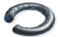
**Description:** The seal exhibits blisters, pits or pocks on its surface. Absorption of gas at high pressure and the subsequent rapid decrease in pressure. The absorbed gas blisters and ruptures the elastomer surface as the pressure is rapidly removed. **Contributing Factors:** Rapid pressure changes. Low-modulus/hardness elastomer.
