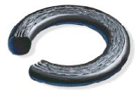
**Description:** The seal or parts of the seal exhibit a flat surface parallel to the direction or motion. Loose particles and scrapes may be found on the seal surface.
