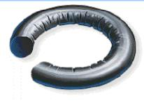
**Description:** The seal may exhibit radial cracks located on the highest temperature surfaces. In addition, certain elastomers may exhibit signs of softening—a shiny surface as a result of excessive temperatures. **Contributing Factors:** Elastomer thermal properties. Excessive temperature excursions or cycling.
