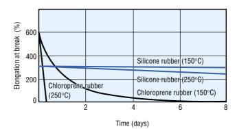
Chloroprene rubber deteriorates rapidly and discolors at temperatures between 150°–250°C, but there is little change in silicone rubber even at 250°C.
