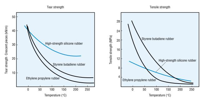
\* The strength of silicone rubber at room temperature is inferior to that of organic rubber,
