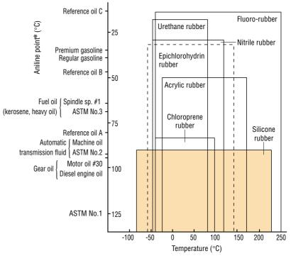
\* Aniline point: the lowest temperature at which equal portions of an oil and aniline are completely miscible. The lower the aniline point, the greater the swelling effect of the oil.
