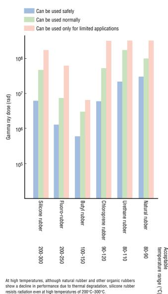
At high temperatures, although natural rubber and other organic rubbers show a decline in performance due to thermal degradation, silicone rubber resists radiation even at high temperatures of 200°C-300°C.
