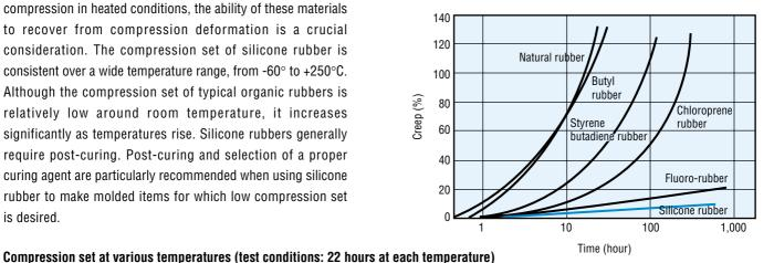
\* Creep is the deformation of a plastic material under constant load. Typically, creep increases as temperature rises. Rubbers that are firm and have greater thermal stability tend to exhibit lower creep values at higher temperatures.
