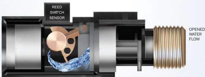
Ⓐ When water flow in, the magnet will be elevated and activate the power sensor to turn on the heater set. (Reed Switch)
