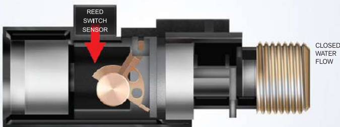
Ⓑ When no water flow in, the magnet will remain and the heater set will not be activated. (Reed Switch)
