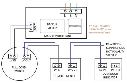
\* Wiring with 0.75/1.0mm2 2-cores alarm cable
