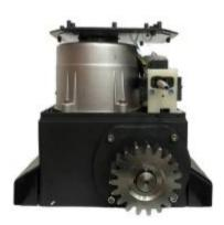
Move the gate manually to the open limit and close limit, mark the points on the rack, then fix the limit stopper or magnets at the limit points on the rack.
