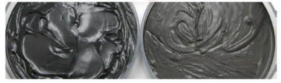
Heat-resistant greases with little tendency to solidify at high temperatures
