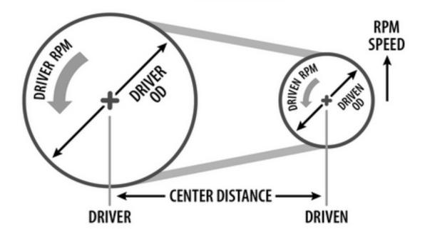
Pulley and belt combination have 98% peak efficiency at the time of installation provided that the allignment and tensioning is perfect.
