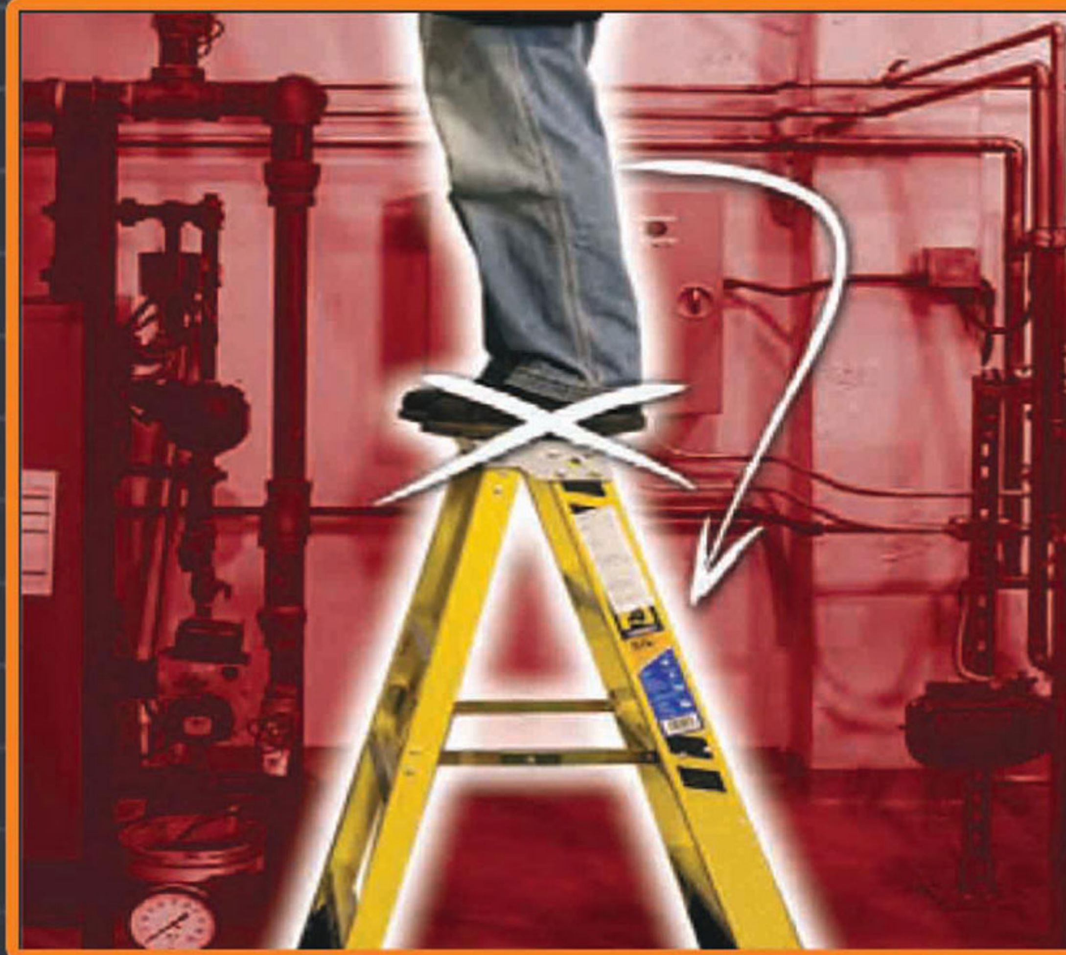
Do not stand or sit on a stepladder top. You could easily lose your balance or tip the ladder. Ladder tops warn users not to stand or sit on them.
