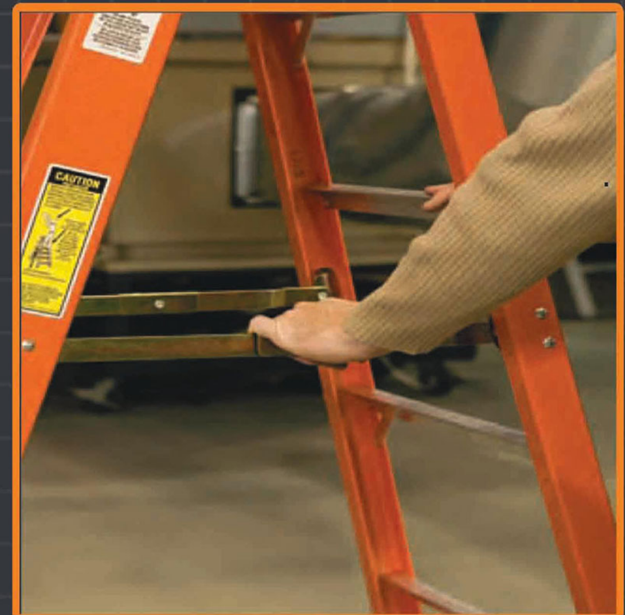
Fully open the stepladder and firmly lock both spreaders.
