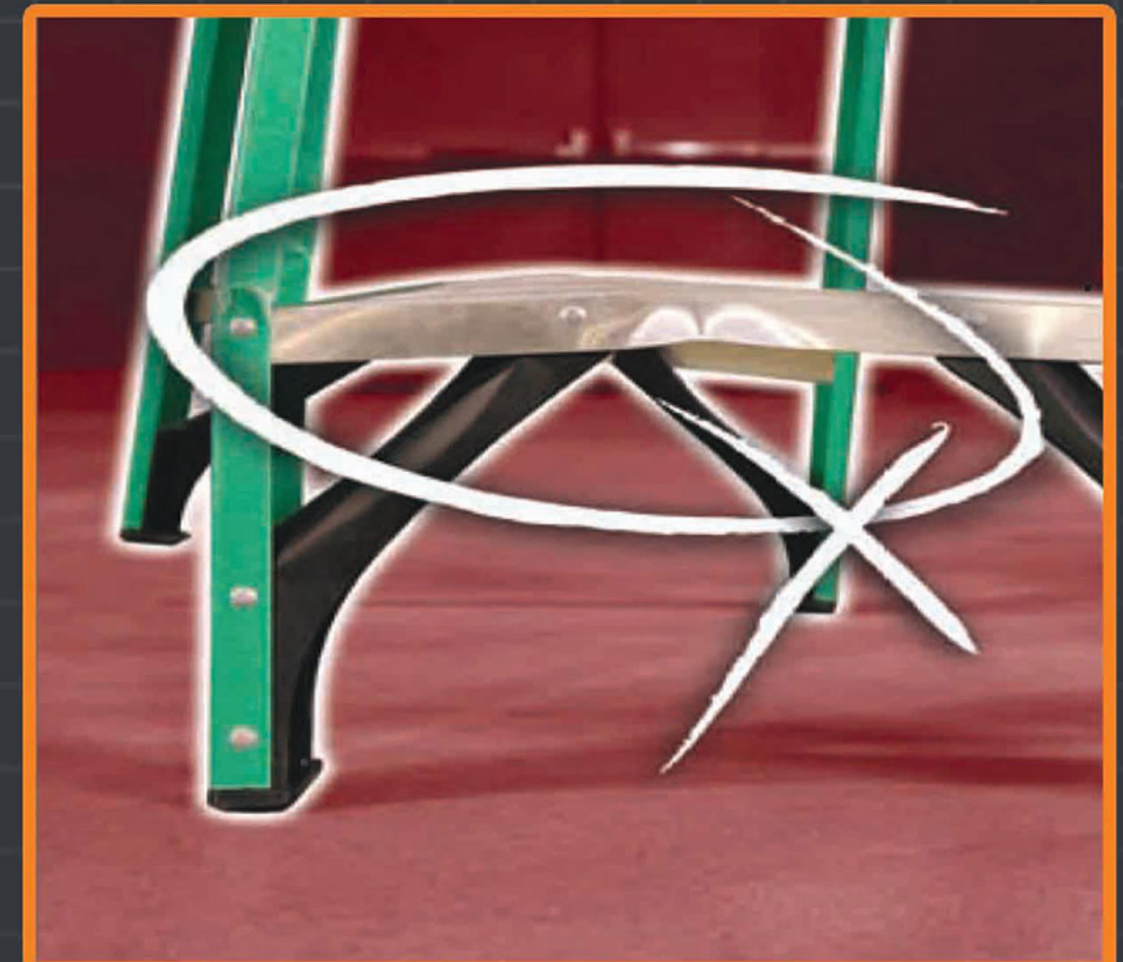
Never use a damaged ladder. Damaged ladders must be tagged for repair or disposal.
