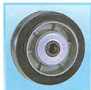
VAE75/100 Rubber (SBR, BR) Aluminium disk Commercial bearing
