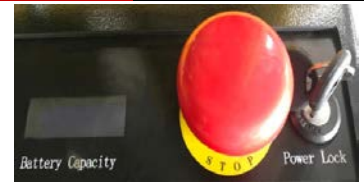
Timer & Emergency Stop switch & Power Switch
