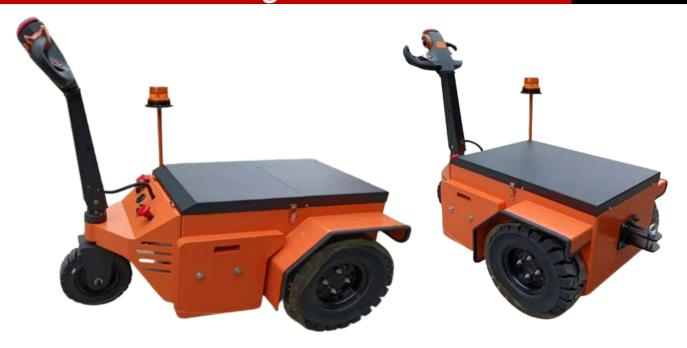
An electric tug is a utility vehicle, which enables the operator to move heavy loads through narrow spaces with ease and safely
