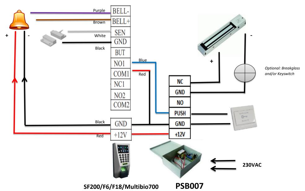
After setting this up, Goto Main Menu > User Management > Access > Access control Parameter > Lock Time 2 sec
