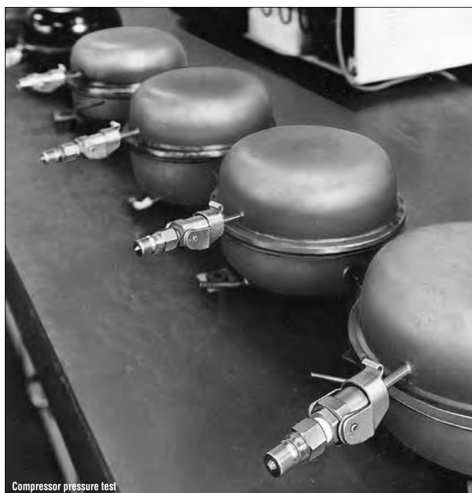
Compressor pressure test
