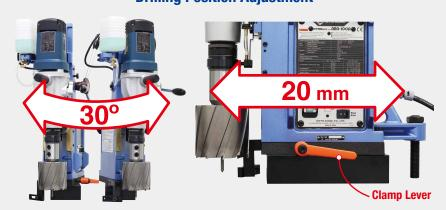
When the clamp lever is loosened, the drill position can be adjusted back and forth by 20 mm and pivoted 15 degrees to the left or right. The clamp lever can be positioned for left hand or right hand operation
