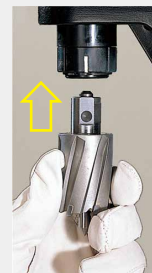
Mounting the cutter
