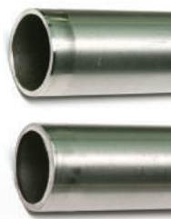
3 Attention : Do not use tube cutter! a) tube cut with tube cutter : heavy burr / bevel cut
