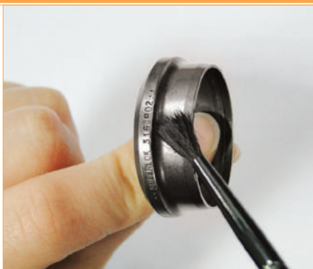
Lubricate thread and cone of fitting body, also compression ring and thread of nut.
