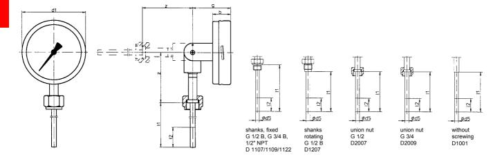
The sensitive portion I2 shall reach the process temperature completely. The insertion length I1 should have adequate size.
