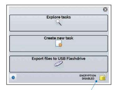
You can create tasks using the touch screen display or by connecting remotely from your computer to the TA. Other methods are also possible such as sending task from your application using our XML description or from an existing Excel™ application. The TA dry block can also pick-up a task directly on a remote server. All these possibilities are described and documented in our communication manual.
