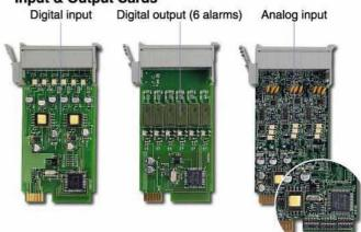
Configure input by DIP switches
