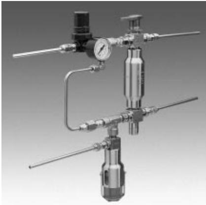
The ability to purge the sample point ensures optimal retrieval of a representative, contamination free sample. The S23 type sampler in continuous needle purge configuration provides a system purge and continuous needle purge in addition to a fixed sample volume.
