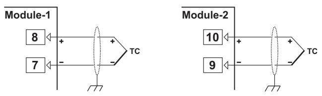
Connect the wires with the polarity as shown above. Always use compensation wire corresponding to the thermocouple used. If present, the shield must be connected to a proper ground.
