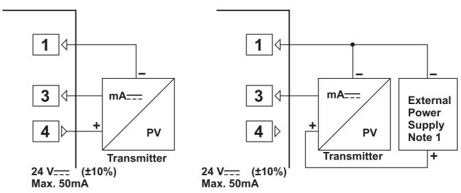
**Note 1:** External power supply must be selected according to supply voltage range and required current for transmitter.
