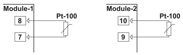
There is no line compensation in PT-100 Input Module EMI-410, EMI-430, EMI-440 or EMI-450 analogue input modules can not be plugged-in Module-1 and Module-2 socket at the same time.
