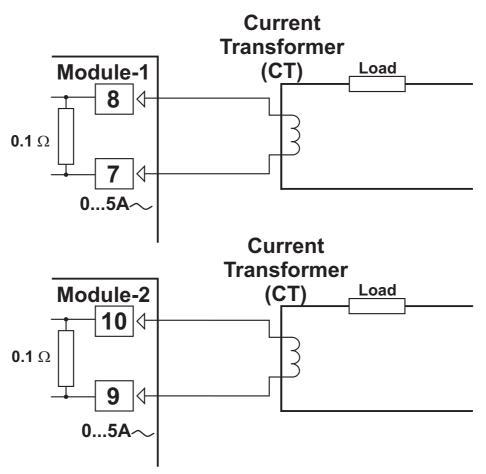
Two EMI-420 ~ CT input modules can not be plugged in Module-1 and Module-2 socket at the same time.
