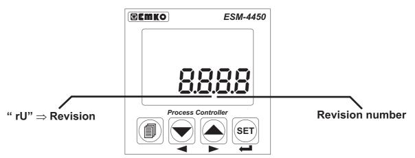
When power on, display of the device is like below:
