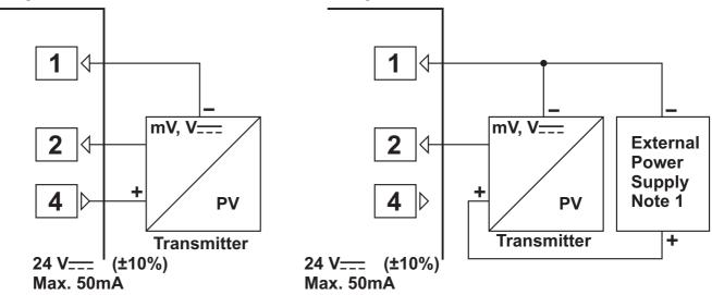
**Note 1:** External power supply must be selected according to supply voltage range and required current for transmitter.
