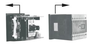
Pull out the cover case from the device
