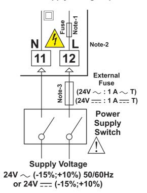
**Note-1**: There is an internal 33R  $\Omega$  fusible flameproof resistor in 100-240 V $\sim$  50/60Hz There is an internal 4R7  $\Omega$  fusible flameproof resistor in 24V $\sim$  50/60Hz , 24V=
