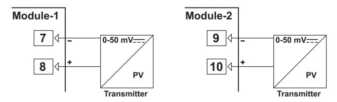
By selecting Module-1 or Module-2 analogue input configuration parameter  $\lceil 5 \rfloor \rceil$  or  $\lceil 5 \rfloor \rceil$  and defining calibration points with dual point calibration property, EMI-430 TC or 0...50mV== module can be used as 0...50mV== input.
