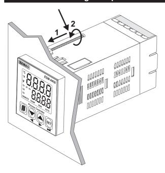
The unit is designed for panel mounting.
