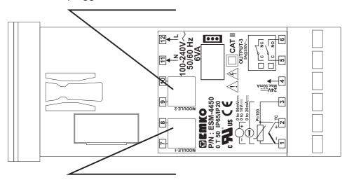
Label which describes terminal connection of module that is plugged in Module-1 socket is attached to this area.
