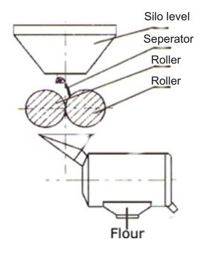
The programming of device should be done according to the operation principles of the milling machine given below.
