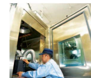
HALT Highly accelerated life test (HALT): Test to confirm the thermal and vibration limits.
