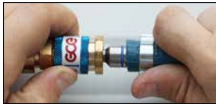
1. Pull the "blue" sleeve of the Quick connector and insert the coupling pin into the Quick connector.
