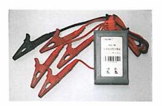
With proper number wireless modules, main tester can real time scan and display the voltage data of each battery during the discharging, and display the histogram of all batteries to follow the battery voltage tracks in whole discharging process.
