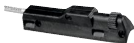
RCC-14 Remote Contactor and Current Control 151086 East/west rotary-motion fingertip control attaches to TIG torch using two hook-and-loop fasteners. Includes 26.5-foot (8 m) cord and 14-pin plug.
