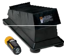
Wireless Remote Hand Control 300430 For remote current and contactor control. Receiver plugs directly into the 14-pin receptacle of Miller machine. 300-foot (91.4 m) operating range.
