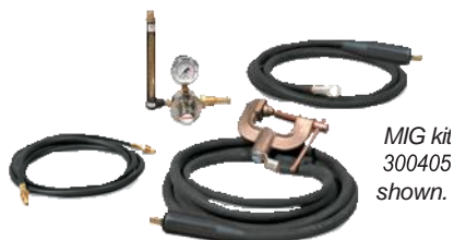
Industrial MIG 4/0 Kit with Dinse Connectors 300405 For single feeders 300956 For dual feeders Consists of flowmeter regulator with 10-foot (3 m) gas hose, 10-foot (3 m) 4/0 feeder weld cable, and 15-foot (4.6 m) work cable with 600-amp C-clamp. Dual kit comes with two flowmeter regulators and gas hoses.
