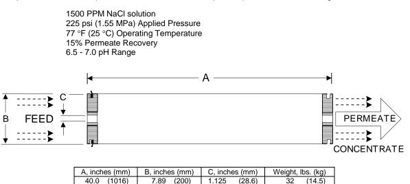
Notice: Permeate flow for individual elements may vary ±15 percent. Membrane active area may vary +/-4%. All membrane elements are supplied with a brine seal, interconnector, and o-rings. Elements are enclosed in a sealed polyethylene bag containing less than 1.0% sodium meta-bisulfite solution, and then packaged in a cardboard box.
