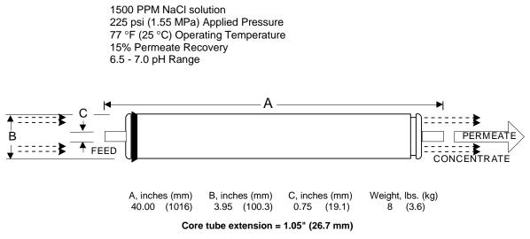
Notice: Permeate flow for individual elements may vary + 33 or - 15 percent. All membrane elements are supplied with a brine seal, interconnector, and o-rings. Elements are enclosed in a sealed polyethylene bag containing less than 1.0% sodium meta-bisulfite solution and 10% propylene glycol, and then packaged in a cardboard box.
