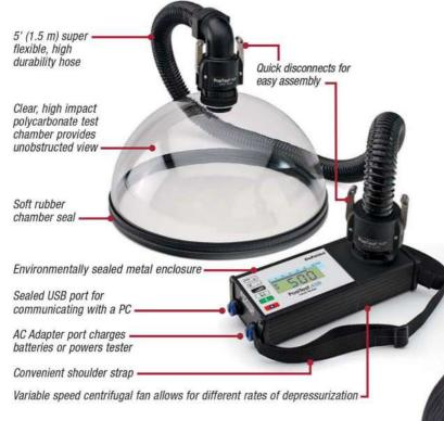
TESTER COMES COMPLETE with shoulder strap, high impact polycarbonate test chamber, durable 5' (1.5 m) hose with quick disconnect couplings, built-in rechargeable NiMH batteries with charger (AC power supply), 8 oz. test solution with dauber (qty. 4), instruction manual, USB cable,
