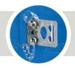
Bubbles indicate an air leak. An estimate of the relative size of the leak can be made based on the size and speed with which bubbles form.
