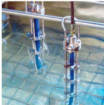
Hydrostatic pressure test
