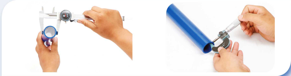
Appearance, dimensions and ovality inspection
