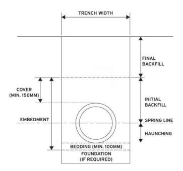
The dimensions of a trench line opening are normally governed by the pipe diameter, method of jointing and site conditions. Normal minimum depth of cover for mains should be 1 meter from ground level to the crown of the pipe.
