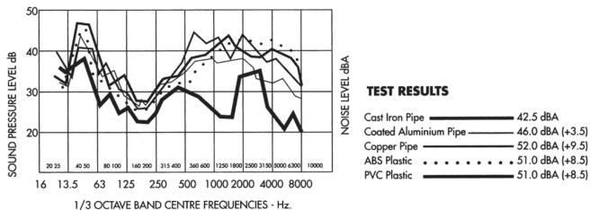
The illustrated chart above shows that cast iron pipe noise level is significantly lower than the other specimens. The "A" scale reading and the differences compared to cast iron pipe are quite significant. A difference of 3 dB is distinctly noticeable. A difference of 10 dB is considered to be doubling subjective loudness. The actual difference in sound power output compared to cast iron is approximately  $2\frac{1}{4}$  times for aluminium, 7 times for plastic and 9 times for copper.
