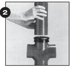
Roll back the gasket, offer the next spigot into position ensuring the central register of the gasket is between the spigots.
