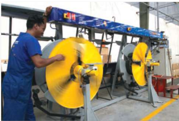
Manufacturing coils on the Buteline Pipewinder
