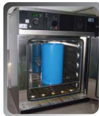
Heat Reversion Test
