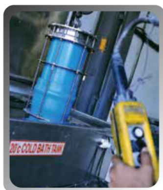
Hydrostatic Pressure Test
