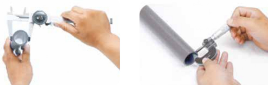
Appearance, dimensions and ovality inspection
