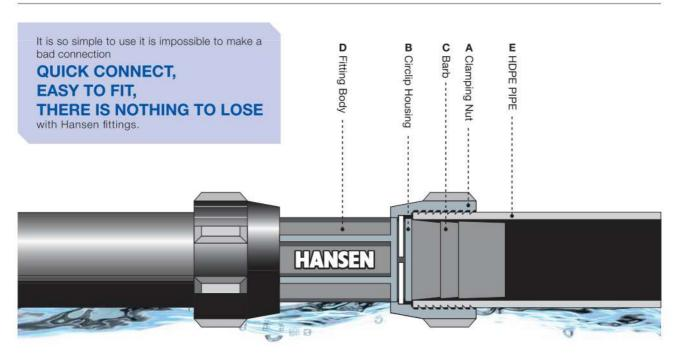
Push the Hansen fitting **D** into the pipe **E** (High Density Polyethylene Pipe) up to the circlip housing **B**.
